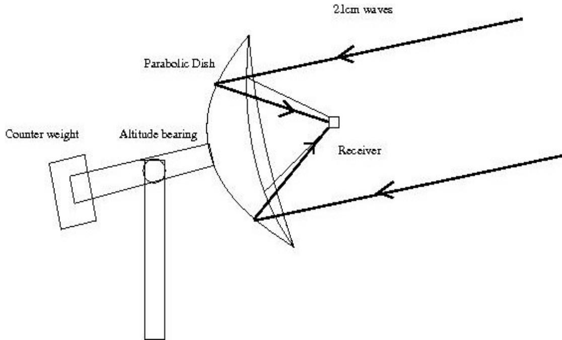
Figure 2. The optical design of the Smiley Radio Telescope
